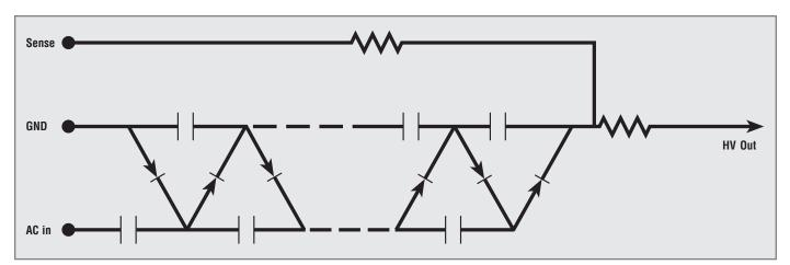
Custom voltage multiplier assemblies for various applications such as CRT, Electrostatic and X-Ray are a major part of our production. Because each application is unique, our engineering staff can help select the elements that will facilitate the operation of each design in the most efficient and cost-effective manner.
