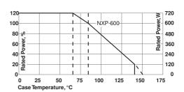
Derating (thermal resist.) NXP 600: 8.33W/°K (0.12°K/W) (for conf. 2, 3) Power Rating: 600W at 85°C bottom case temp.\*
