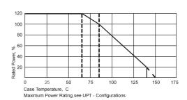
Derating (thermal resist.) UPT 600: 8.33W/°K (0.12°K/W) (for conf. 2 and 3)
