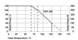
Derating (thermal resist.) UXP 300: 4.35W/°K (0.23°K/W) Power Rating: 300W at 85°C bottom case
