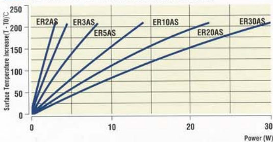
Fig. 4 AS Power vs. Surface Temperature Increase (1)
