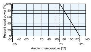
For resistors operated at an ambient temperature of  $70^{\circ}\!\mathrm{C}$  or higher, the power shall be derated in accordance with the above derating curve.
